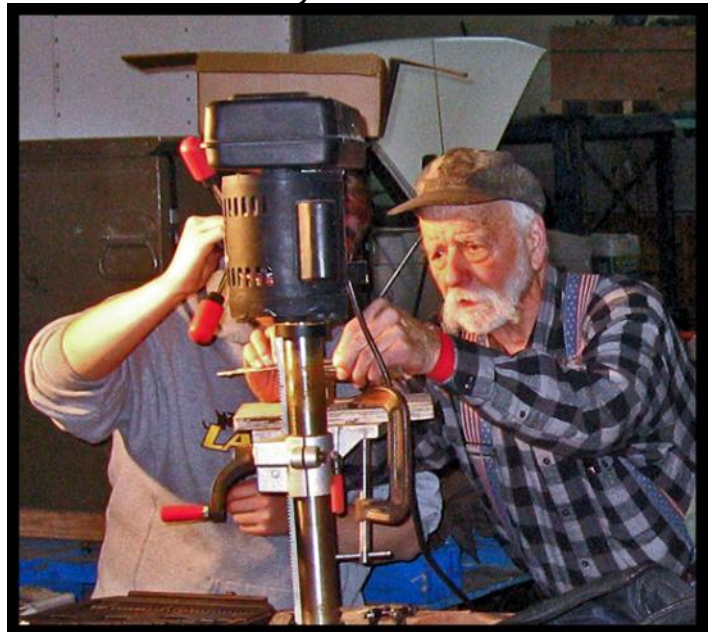
Wind Drifter helps Sure Shot Chris line up his knife project for drilling the holes for handle pins during Saturday's inaugural knifemaking class. Photo: Valencia Rose.
